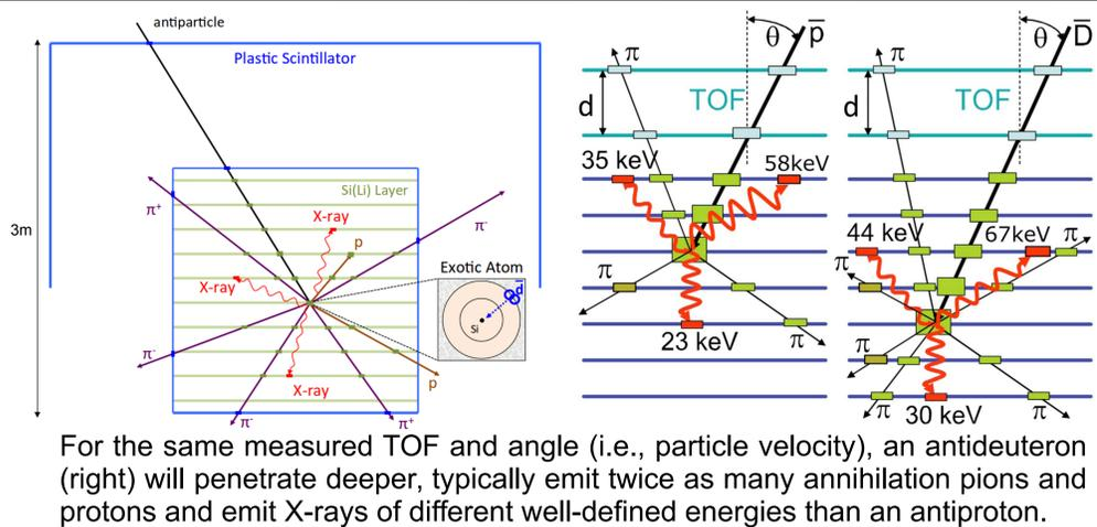
For the same measured TOF and angle (i.e., particle velocity), an antideuteron (right) will penetrate deeper, typically emit twice as many annihilation pions and protons and emit X-rays of different well-defined energies than an antiproton.
