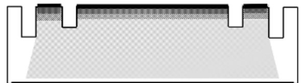
(e) Cut guard ring groove and re-apply contacts
