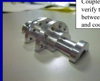
Coupler test model to verify the heat coupling between detector holder and cooling pipe
